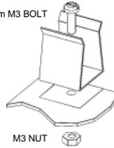
Mount the battery clip on the PCB using the 4mm M3 bolt and M3 nut.
