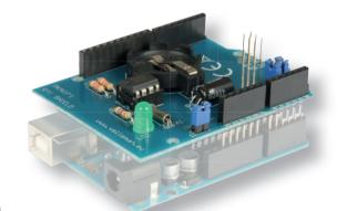
Add a real time clock shield to your projects to ensure accurate and easy timekeeping. While the shield keeps track of time and date, the controller can focus on other tasks.
