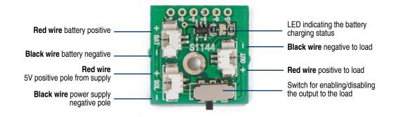
The charging current (Ireg) is set by the resistance connected to pin 5 (R1 in our case). The current value is reckoned as follows: Ireg = 1000 / R
