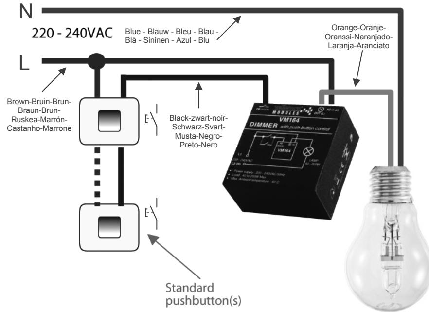
**UK** Use the standard pushbutton to set a dimming light intensity and to create a suitable atmosphere.
