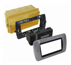
The sensor (VMB1TS) can be build-in together with a controller (VMB1TC) in a 4-module wide frame with cover plate from the BTicino Light of Light Tech series. The module must be pushed into the build-in frame from the front
