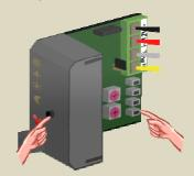
6. Press and hold the pushbutton on the front panel of the second sensor module and simultaneously press and hold the lowest push button (HEAT) until the relay is energised and the red LED on the sensor module flashes. First release the lowest push button (HEAT) followed by the push button on the front panel.
