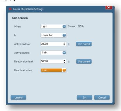
The three conditions are now set. The output channel "Sunscreen" (CH3) will close when one of the conditions is met. It will only open when none of the conditions are met.
