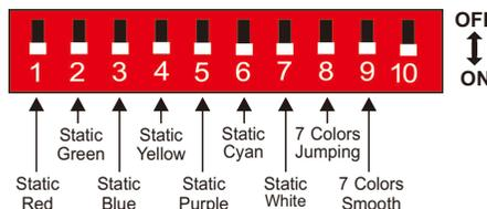
For changing effects (Dip Switch 8/9=ON): DIP switch 1-7 is used to realize 7 speed levels. (7=ON, the fastest level)
