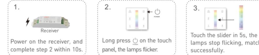
Method 2 : When the touch panel is on and the wiring between the receiver and the lamps are correct.
