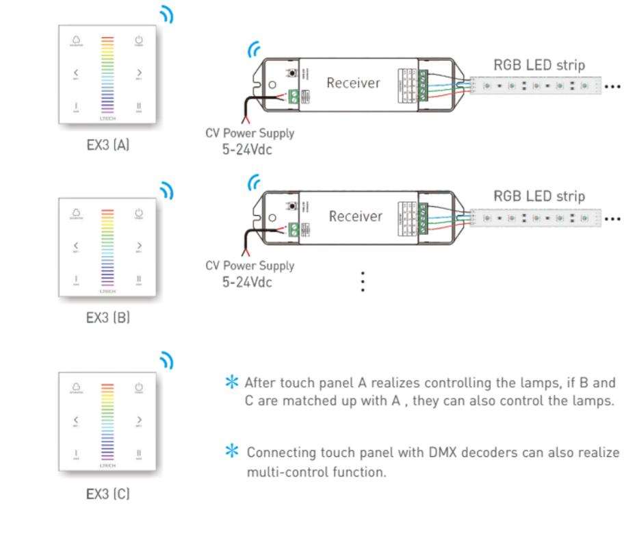
\* After touch panel A realizes controlling the lamps, if B and C are matched up with A, they can also control the lamps.
