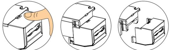
Pull the housing left and right from the bottom to remove it.
