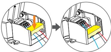
Push the tension plate down to fix the electric wire.
