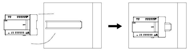
1. Fix the DIN rail onto the wall.
