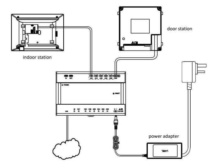
Wire the devices with power supply cables as picture shown.
