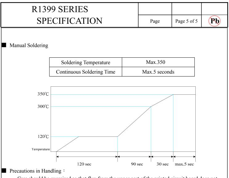
Care should be exercised so that flux from the upper part of the printed circuit board does not adhere to the switch.
