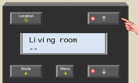
7. Confirm with the → button. The program instruction is removed from the memory, the flashing cursor disappears and the next program instruction is shown. If this was the last instruction, the display remains empty.
