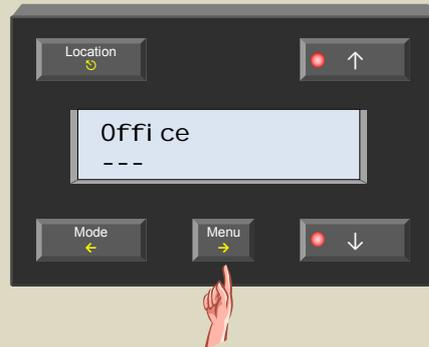
19. Select the sensor in the passage (to set up the differential thermostat) with the ↑ or ↓ button.
