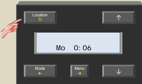
10. Now set the addresses of all shutter modules to 'E2' to learn the immediately up action for channel 2. The 'Mode Up2' LEDs are flashing to indicate the learning mode.
