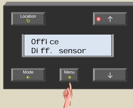
21. Scroll through the sensor settings menu using the ↑ or ↓ button until the 'Temp difference' item appears.
