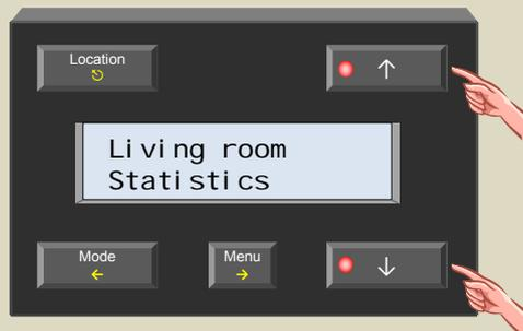
4. Select the statistics menu with the → button. The display shows the minimum temperature.
