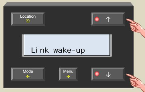
15. Select the link wake up menu with the → button. As a confirmation, the relays of the window shutter modules are energised.
