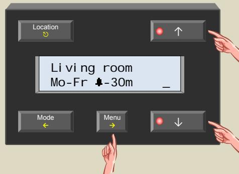
9. Set the mode (comfort, day, night or anti-freeze mode) with the ↑ or ↓ button and confirm with the → button.
