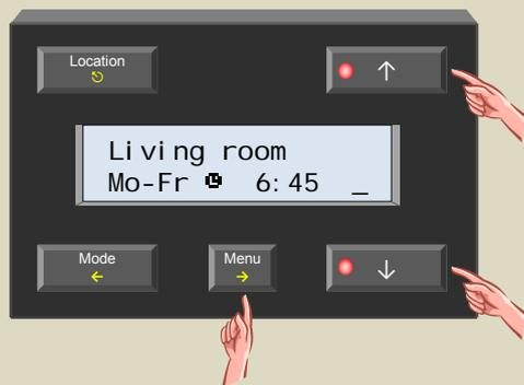
10. Set the mode (comfort, day, night or anti-freeze mode) with the ↑ or ↓ button and confirm with the → button.
