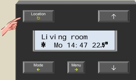
2. Press and hold the 'Menu' button for  $\pm 4$  seconds to open the extended menu. Enter the PIN code if necessary.
