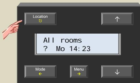
2. Set the heating (or AC) to anti-freeze or night mode using the 'Mode' button.
