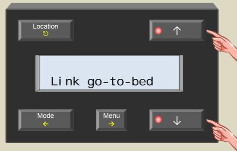
7. Select the link go to bed menu with the  $\rightarrow$  button. As a confirmation, the relay of channel 1 is energised.
