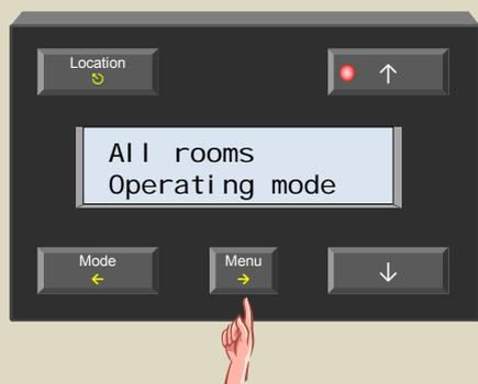
5. Scroll through the sensor settings menu using the ↑ or ↓ button until the 'Unjam valve' item appears.
