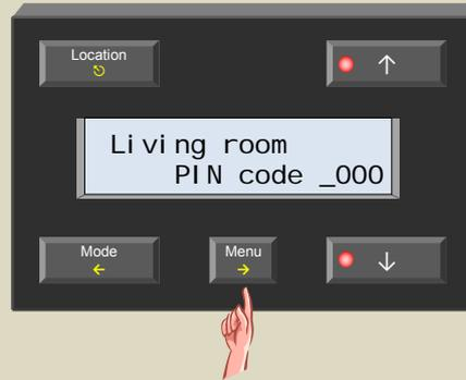
6. Change the first number of the PIN code with the ↑ or ↓ button and confirm with the → button.
