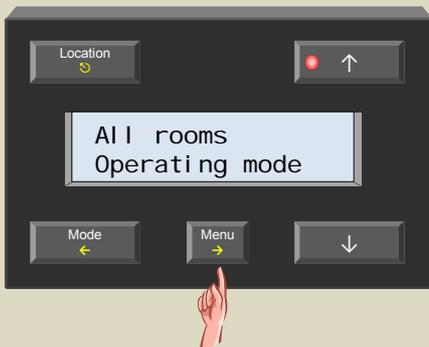
5. Scroll through the sensor settings menu using the ↑ or ↓ button until the 'Upper cool temp' item appears.
