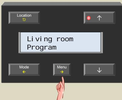
4. Scroll through the extended menu using the ↑ or ↓ button until the 'Sensor settings' item appears.
