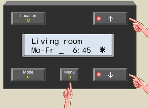
7. Use the ↑ or ↓ button to set the time reference (exact, relative to wake-up or go-to-bed time) on which the instruction needs to be executed. Confirm with the → button.
