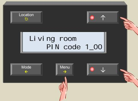
7. Change the second number of the PIN code with the ↑ or ↓ button and confirm with the → button.
