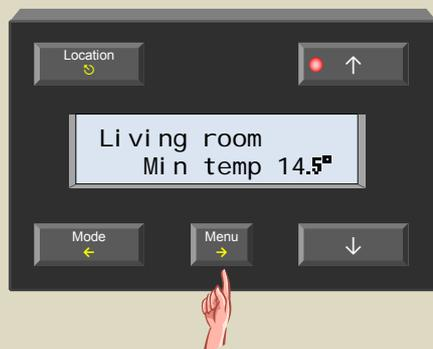
5. Scroll through the statistics menu using the ↑ or ↓ button until the statistic appears that needs to be reset.
