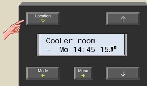
**Set the sensor of the bedroom to cooling mode via the temperature controller**
