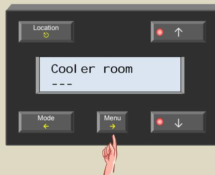
7. Select the second sensor of the differential thermostat using the ↑ or ↓ button.
