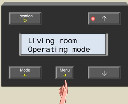
5. Scroll through the sensor settings menu using the ↑ or ↓ button until the 'Temp calibration' item appears.
