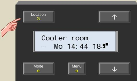
8. Press and hold the 'Menu' button for ±4 seconds to open the extended menu.
