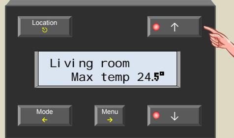
6. Press the  $\uparrow$  button. The first time indication shows how long the heating or AC was on during anti-freeze mode. The second time indication shows how long anti-freeze mode has been enabled.
