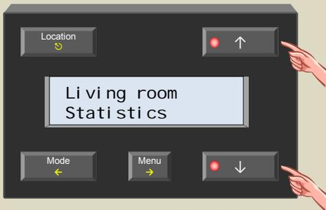
4. Select the statistics menu with the  $\rightarrow$  button. The display shows the minimum temperature.
