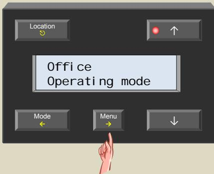
17. Scroll through the sensor settings menu using the ↑ or ↓ button until the 'Diff. sensor' item appears.
