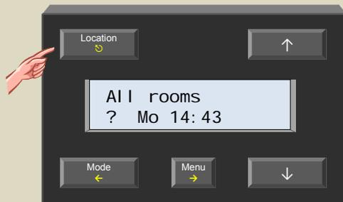
2. Press and hold the 'Menu' button for ±4 seconds to open the extended menu.
