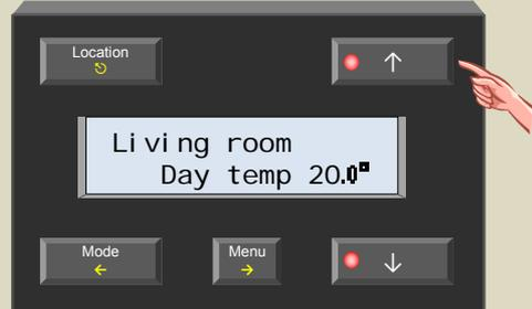
8. Select the day item with the → button. The desired daytime temperature starts flashing.
