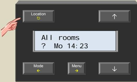
2. Set the heating to anti-freeze mode using the 'Mode' button.
