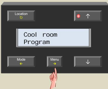
9. Scroll through the extended menu using the ↑ or ↓ button until the 'Sensor settings' item appears.
