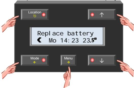
The battery voltage watchdog must be enabled through the configuration menu.
