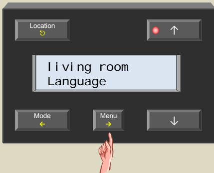
4. Scroll through the configuration menu using the ↑ or ↓ button until the 'Firmware version' item appears.
