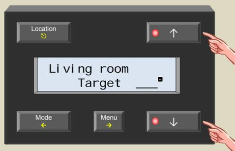
2. When desired, change the target temperature with the ↑ or ↓ button.
