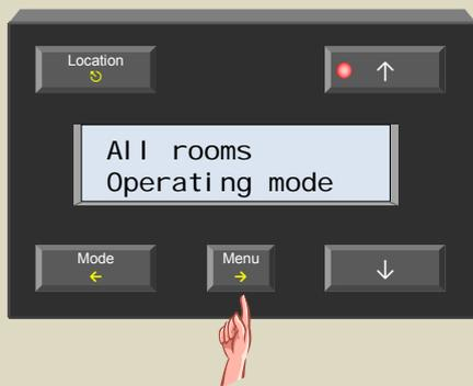
5. Scroll through the sensor settings menu using the ↑ or ↓ button until the 'Unjam pump' item appears
