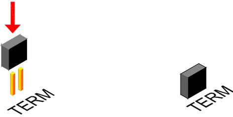
On all other modules, the terminator must be removed.
