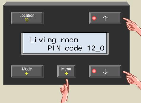
8. Change the third number of the PIN code with the ↑ or ↓ button and confirm with the → button.
