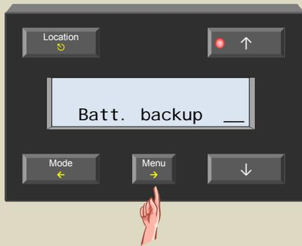
6. Enable the battery backup watchdog when a battery is inserted or disable it when no battery is present using the ↑ or ↓ button.
