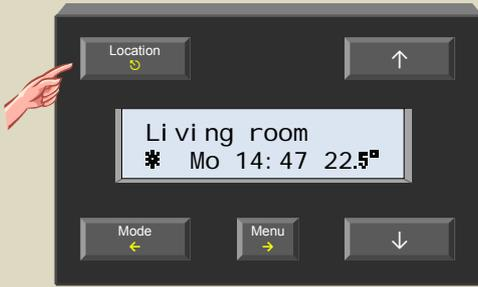
2. Press and hold the 'Menu' button for ±4 seconds to open the extended menu. Enter the PIN code if necessary.
