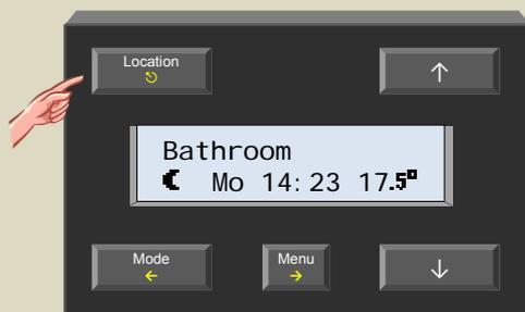
2. Press the 'Mode' button (bottom left) multiple times until the desired mode (-⌚, 🌙⌚, ☀️⌚ or 🛋️⌚) is displayed.
