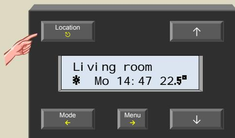
2. Press and hold the 'Menu' button for ±4 seconds to open the extended menu. Enter the PIN code if necessary.
