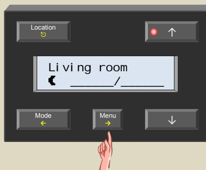
7. Use the ↑ or ↓ button until horizontal lines are displayed in the data entry fields.
