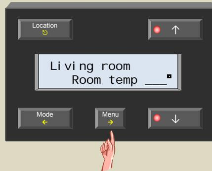
7. Enter the temperature as measured with a different thermometer using the ↑ or ↓ button.
