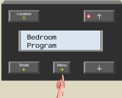
22. Scroll through the extended menu using the ↑ or ↓ button until the 'Sensor settings' item appears.
