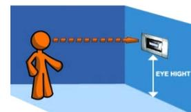
Install the controller at eyesight level!
