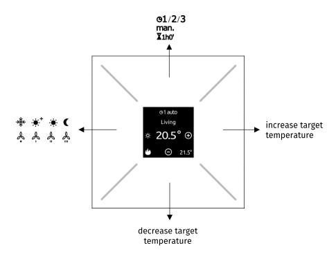
• pressing the left button changes the mode of the thermostat (day/night/comfort/anti-frost in heating mode, or mode I/II/III/standby in airco mode)
