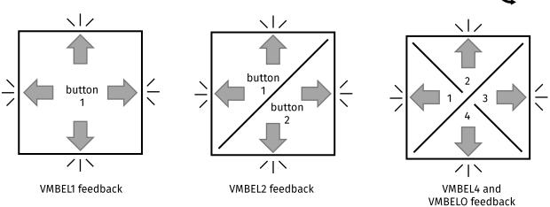
Feedback lighting has priority over ambient lighting. If you want to have only ambient lighting which is not disturbed by feedback lighting, set all feedback to "no feedback" (see "Example 1: only ambient, no feedback" below).
