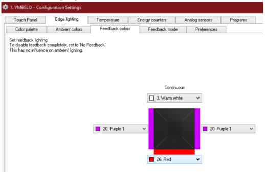
You can choose a different feedback color for each side (and in addition, on VMBELO modules, for each page), and if you wish, also for continuous, slow and fast blinking feedback (check the "advanced settings" checkbox on the feedback configuration tab).
