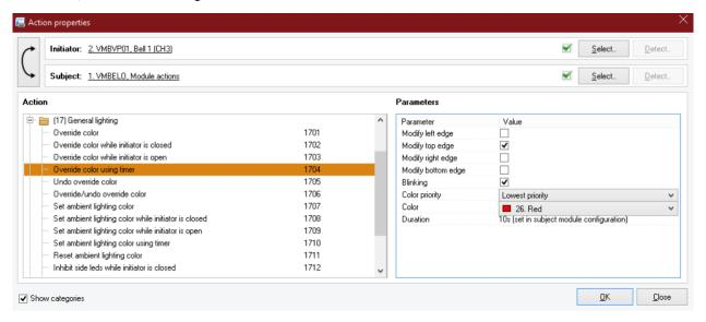
The duration of the timer of action 1704 (and other lighting actions involving a timer) is not set in the action parameters, but in the <u>subject</u> module's configuration settings:
