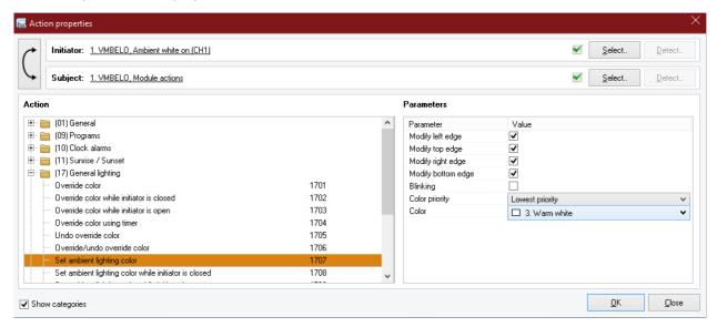
By pressing button 1 "Ambient white on" the ambient lights will be turned on with the color warm white. Button 2 will turn the ambient lighting on with the color red, and button 3 with the color blue. By pressing button 4 "Ambient off" the ambient lights will be turned off. These actions will have no effect on the feedback lighting.
