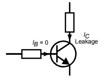
Leakase current Ic=0.17mA Older Germanium types however can suffer from significant collector leakage current, particular at high temperatures (leakage current can be <u>very</u> temperature dependant).
