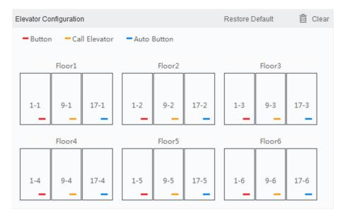
Figure 15-11 Relationship between Relay and Floor
