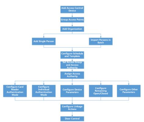
Figure 15-1 Flow Chart of Access Control
