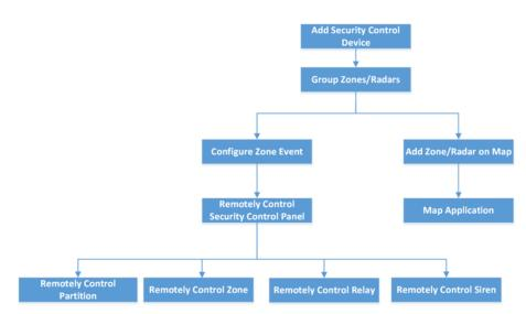
Figure 13-1 Flow Chart of Security Control Panel
