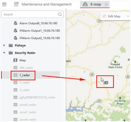
Figure 9-14 Drag a Security Radar to the Map
