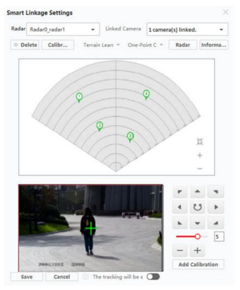
Figure 9-27 Multi-Point Calibration Radar Page
