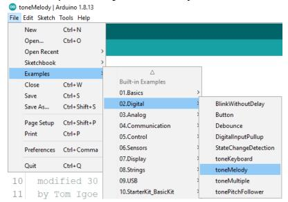
2. Connect your Arduino compatible board, make sure the correct Board and connection port are set in the tools menu, and hit Upload
