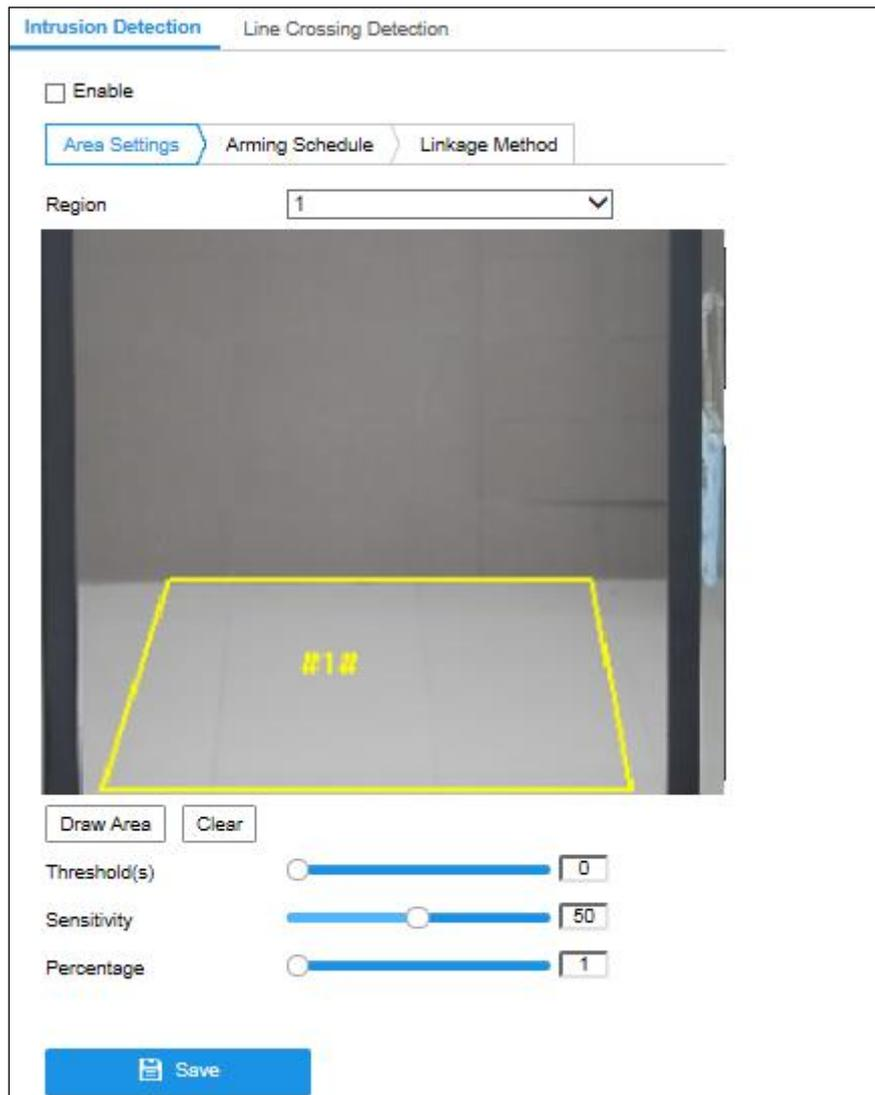
Figure 10-12 Intrusion Detection
